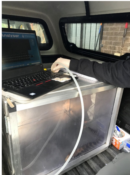
Figure 2. NOS.E analysis using live reptiles. The sensor response was determined not to be reptile specific. This supports that further research must be completed in order for more specific sensors to be selected and installed into the NOS.E.
