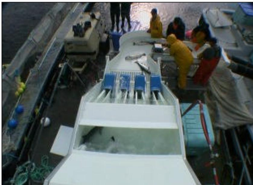
**Figure 1** SI-5 Pneumatic Auto Stunning System in operation in Canada (picture supplied by [www.seafoodinnovations.com.au](http://www.seafoodinnovations.com.au))
