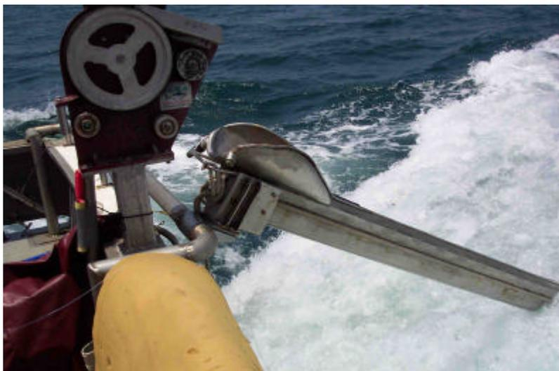
**Figure 3** The underwater bait setting chute is helping to reduce the toll on seabirds in the tuna fishery
