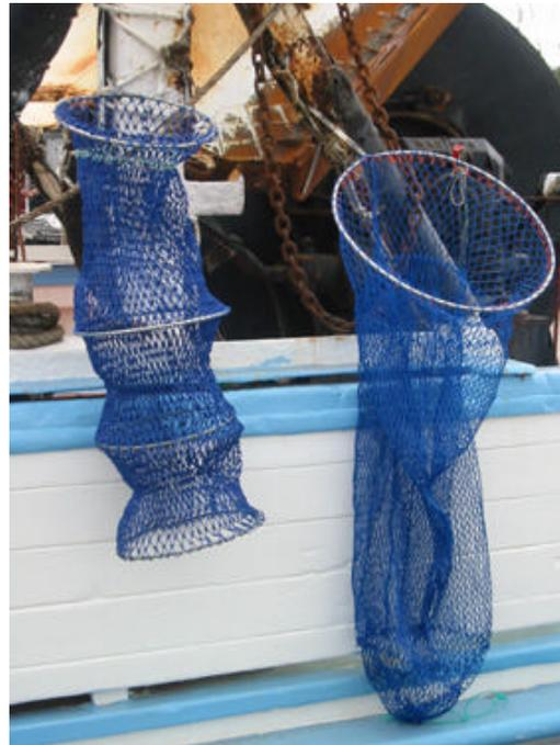
**Figure 2** The simple (left) and cod-end (right) versions of the underwater discard chute
