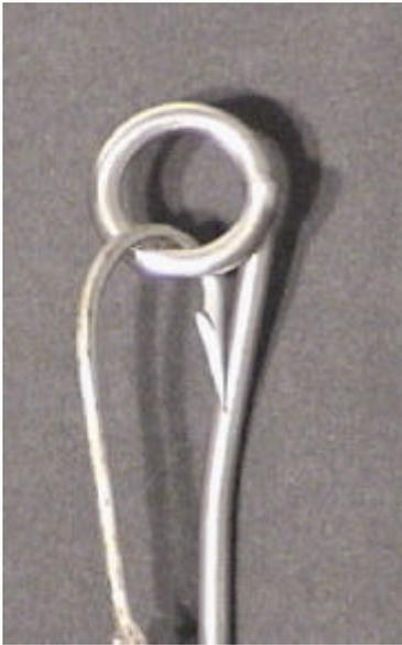
**Figure 4** The head of a de-hooker (note how the barb is protected by the offset bend)
